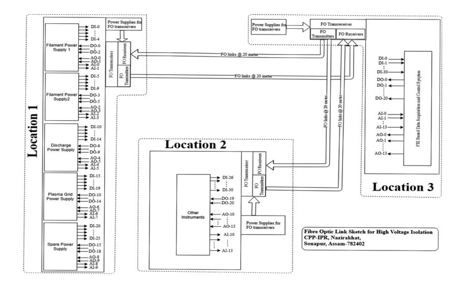
Fig. 1. Block diagram of fibre optic links
